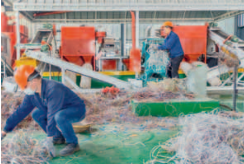
Workshop (5) Workers putting wires into copper granule machines 工作間(5)工人將電線放入銅米機
