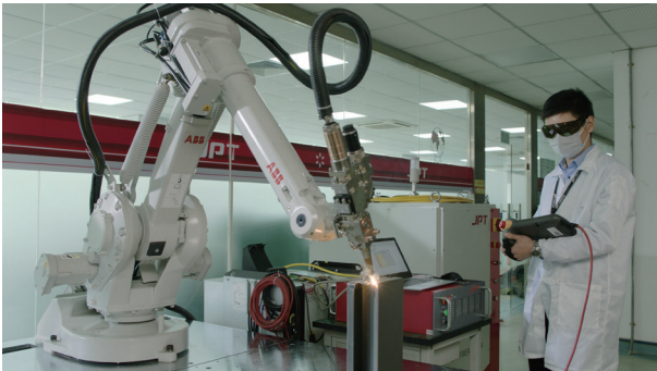
Welding application test of JPT CW laser in cooperation with robot arm
