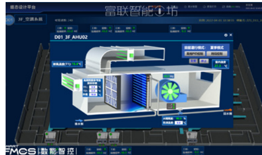
Operation Screen of Air-conditioning System
