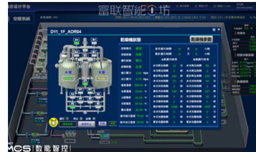
Operation Screen of Dryer
