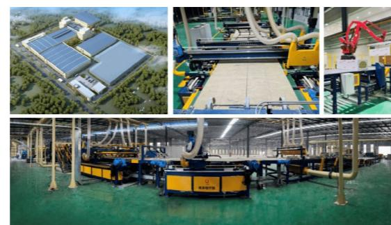
Compared with the traditional rock wool production line, the comprehensive energy consumption of rock wool production line in electric melting method has been reduced by more than 40%. The proportion of solid waste to replace ore has reached 70%, and the emission of melting waste gas has been reduced by 90%. The comprehensive technology has reached the international advanced level, assessed by the China Building Materials Industry Association.
