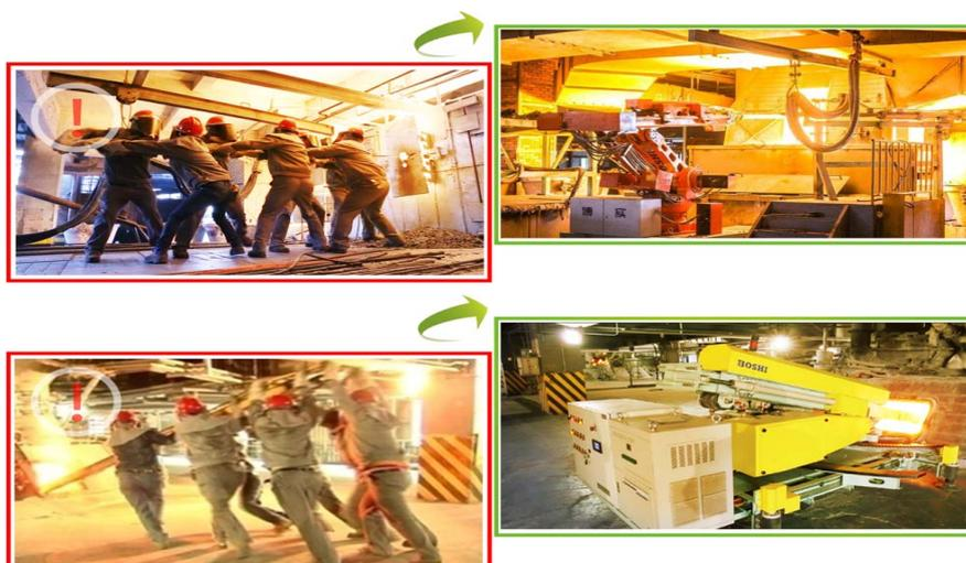
Legend: Schematic diagram of Sub-merged arc robot and tamping robot replacing manual operation replacing manual operation
