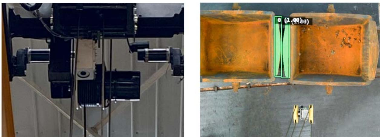
Using deep learning technology, AI recognizes the position and status information of carbide pot trolley, and intelligent crane realizes intelligent lifting and loading of calcium carbide pot with the help of anti-rocking technology.
