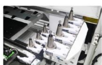
八刀位自动换刀刀库 ATC 8 by servo
