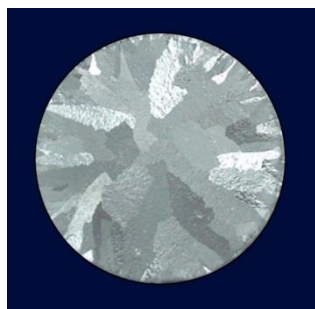
细化前晶粒形态 (20mm)
