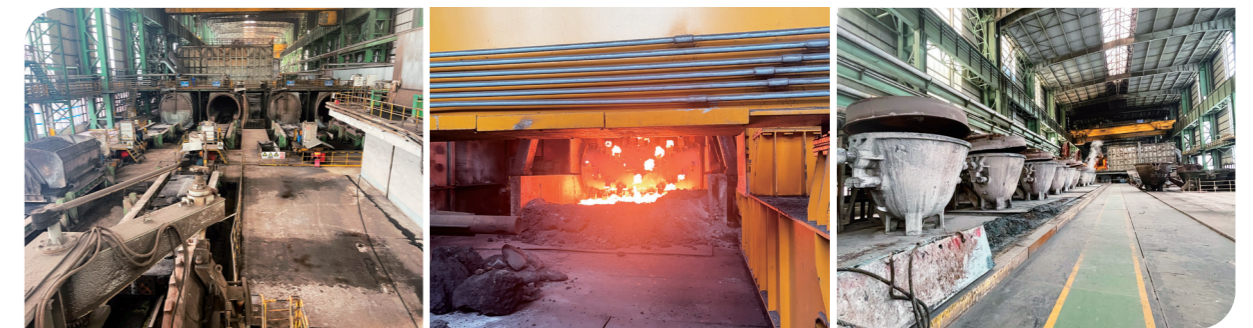
Steel slag roller press + pressure-hot stew processing line
