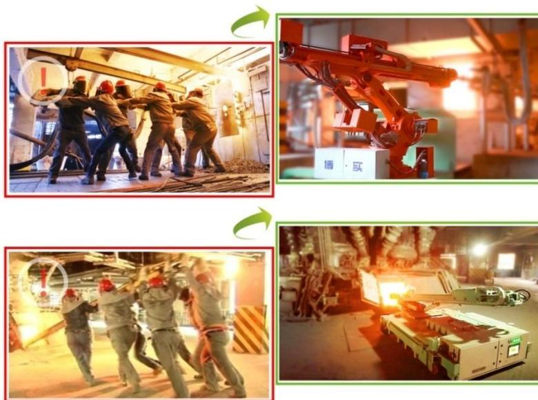
Legend: Schematic diagram of Sub-merged arc robot and tamping robot replacing manual operation replacing manual operation
