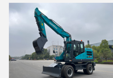
拥有两节动臂的轮式挖掘机SWE155FW
