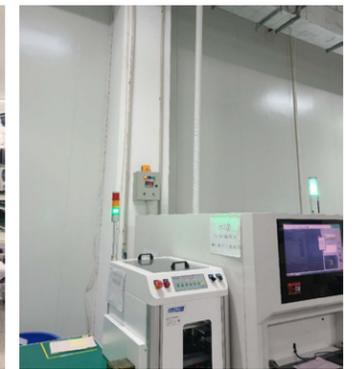
Laser Engraving Exhaust Gas Collection Devices
