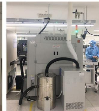
Installation of Dust Removal Devices on Cutting Machines
