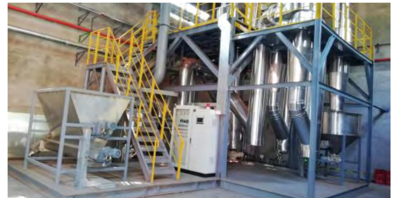
Pilot equipment for drying and pyrolysis of brewing waste
