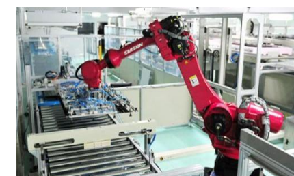
Automatic backlight module production line
