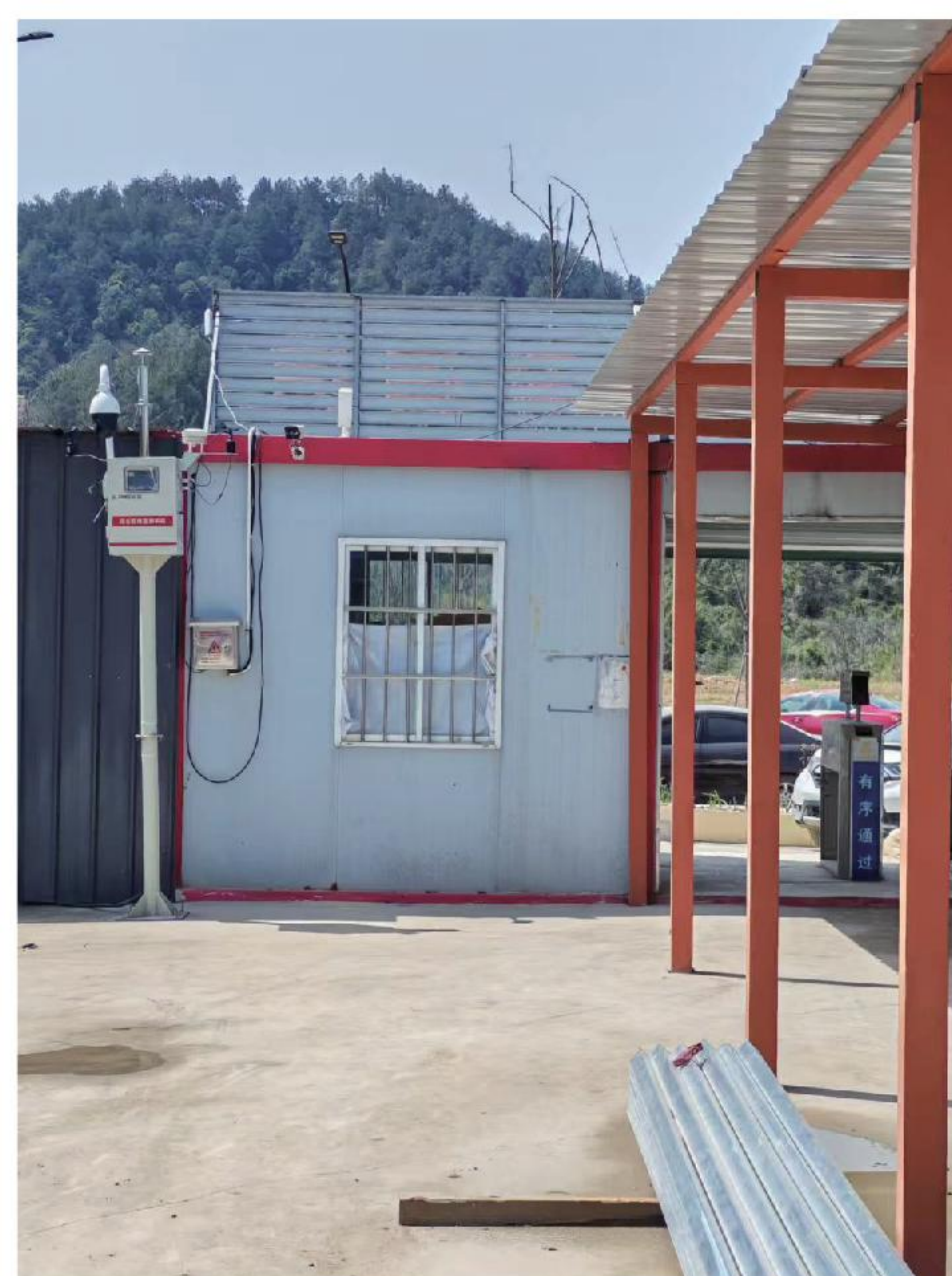
Figure: Installation of an online dust concentration monitoring device
