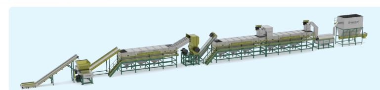
In 2024, to address the challenge of processing large volumes of PE drip irrigation tape waste in agriculture, the Company developed an integrated process combining pre-washing, crushing, scrubbing, rinsing, and dewatering. This solution significantly increased cleaning efficiency to 2t/hour. Together with an advanced water circulation system for sediment filtration and water reuse, it greatly reduced water consumption and improved the quality of subsequent pelletizing.
