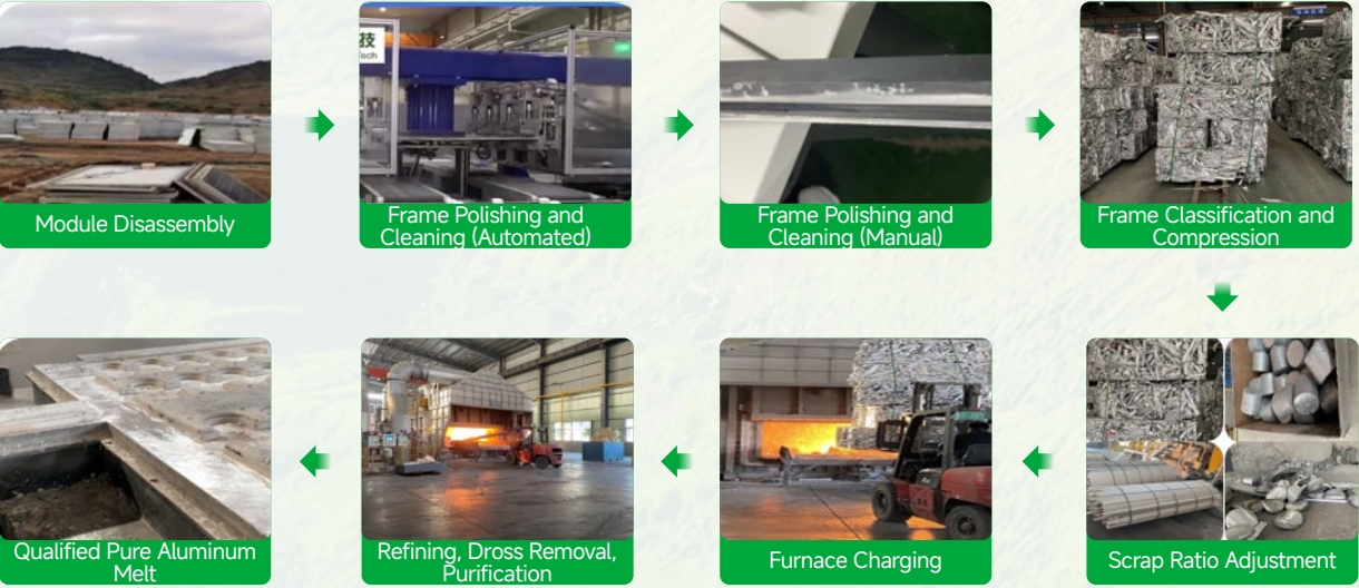
▲ Pre-casting Treatment Process for End-of-Life Module Frames
