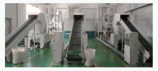
Defective Injection-Molded Products Crushed into Plastic Particles in the Powder Room and Reused in the Injection Molding Machine's Material Loading Area
