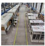
The fire-fighting equipment and fire exit Pedestrians and logistics vehicles are not separated in the workshop aisles
