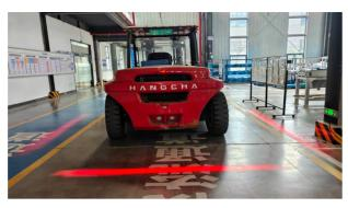
Forklift Equipped with Distance Alarm and Zone Warning Lights
