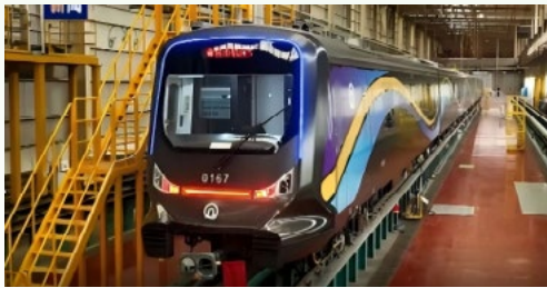
The first carbon fiber subway train in the country, CETROVO 1.0 - Carbon Star Express Rail
