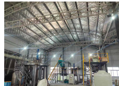
Experimental platform for collaborative disposal of waste incineration fly ash and silicon-rich waste
