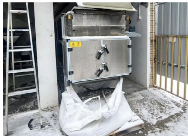
A newly purchased sludge drying machine has been deployed to reduce sludge volume
