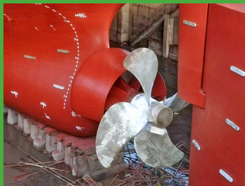
Duct and Propeller Cap Fins on the "Egert Oasis"
