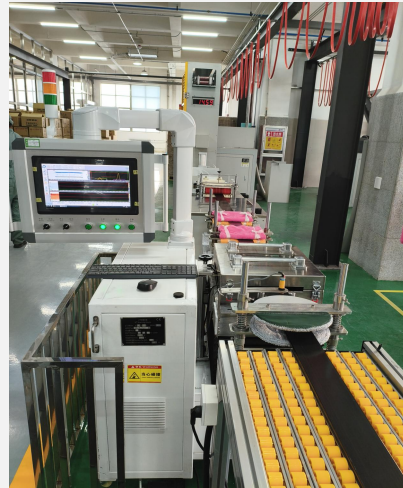
▲ Automated Non-destructive Testing System for Carbon Planks
