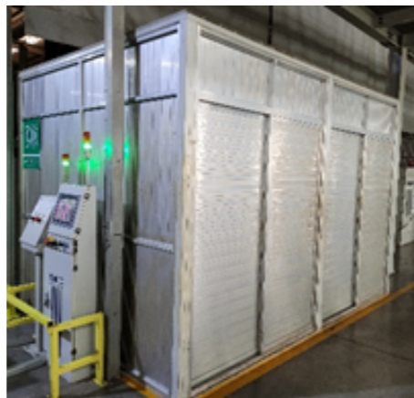
Containment Management of Noise Sources
