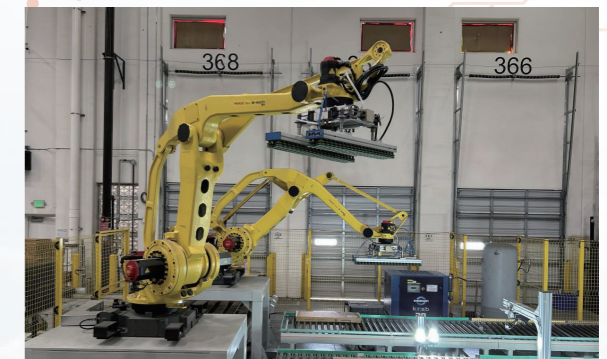
Robotic Arm Depalletizing, Palletizing and Labeling Assembly Line
