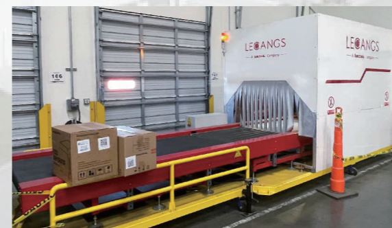
Automated Equipment - DWS System
