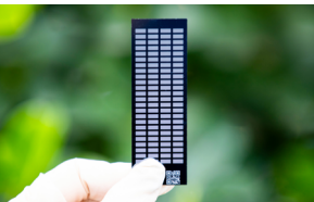
The Xinxiwang 60K High-Density Solid-Phase SNP Chip
