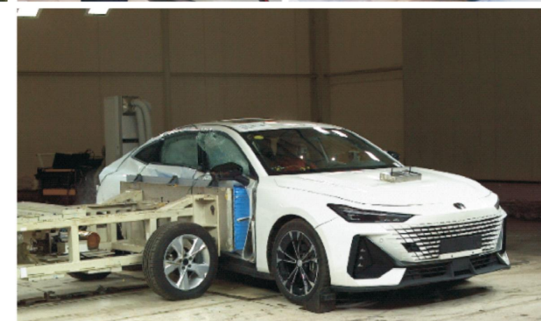
正面、侧面、带角度及追尾碰撞安全性能验证 Safety performance verification of frontal, side, different angles and rear-end collision
