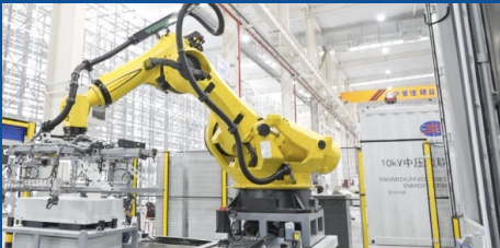
Automatic clustering production line in the Energy Storage Digital Factory
