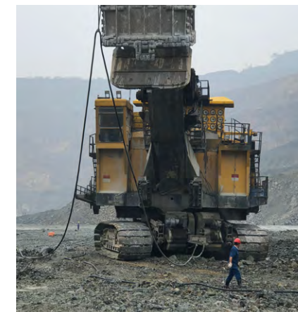
铺设矿山用高柔性高耐磨电缆
