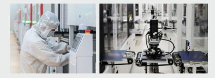
The module production workshop: adopt intelligent production line and automatic optical inspection and judgment equipment (based on AI technology) to detect the defects of module products visually and replace the traditional manual detection, enhancing the test efficiency and improving product yield. Intelligent production line equipment has adopted precise positioning welding solutions and achieved millimeter-level precision positioning required for MBB module production.
