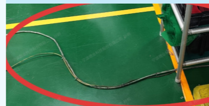
Lack of protective measures for wiring
