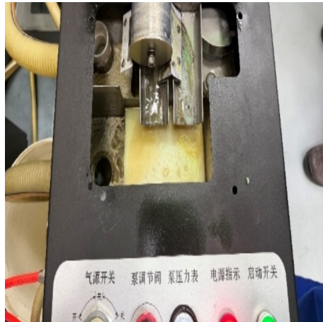
CNC equipment fitted with an oil-water separator
