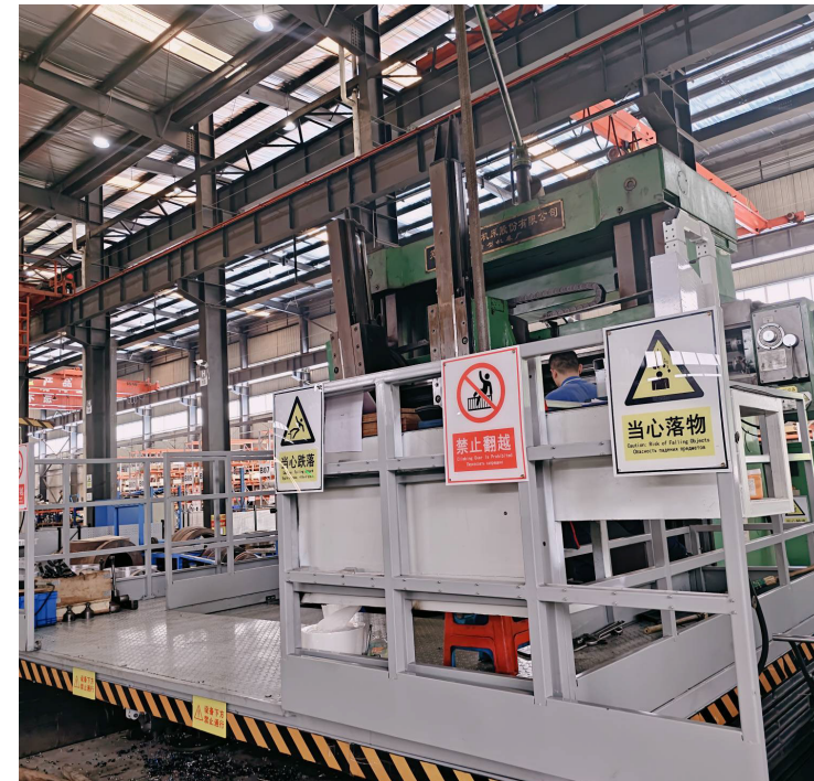
The upgraded vertical lathe operating platform
