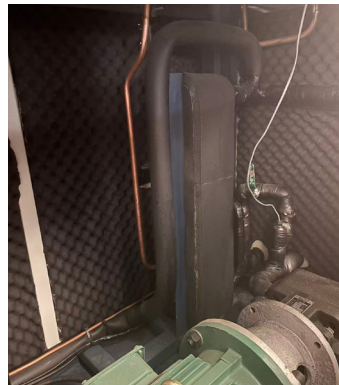
Sound-absorbing cotton on the test bench in Sun Seals’ production department
